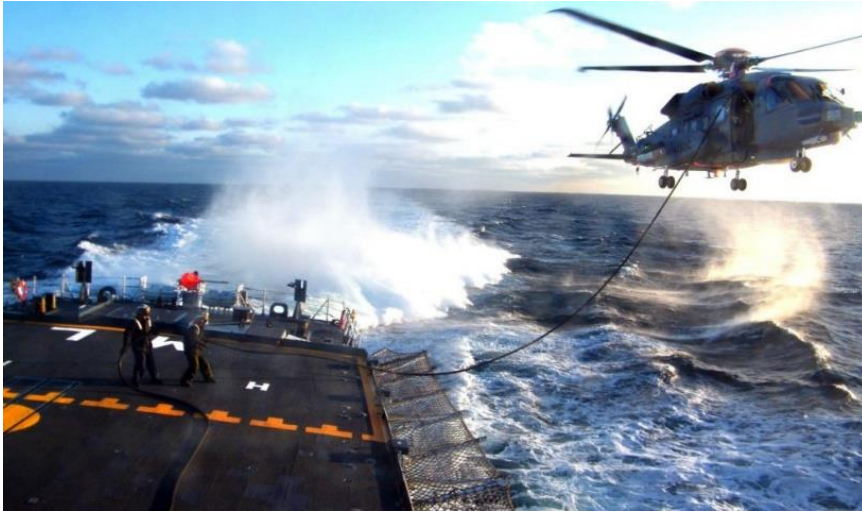
A Cyclone is pictured performing a hover-in-flight refueling test during sea trials aboard HMCS Montréal.
