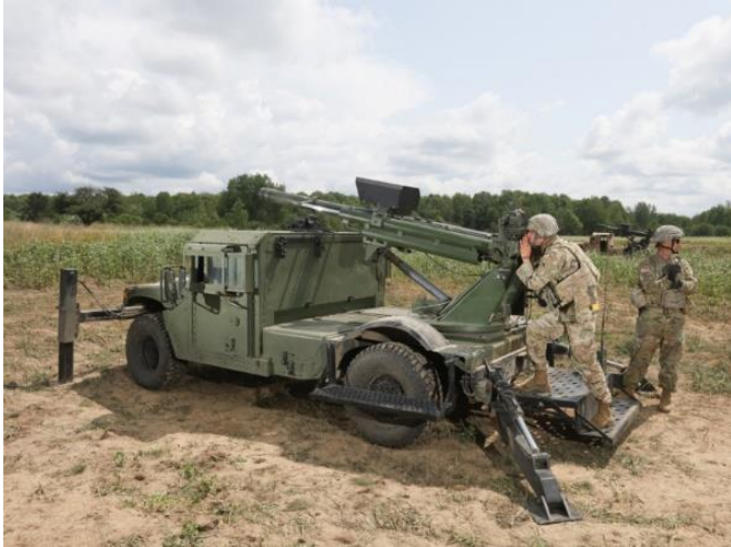
Hawkeye is a light-weight mobile weapon system based on Humvee vehicle.
