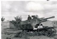
chassis was a German modification of the French-made Lorraine 37L chassis from all those captured during the 1940 campaign. This is a very rare vehicle as most of the Lorraine Schlepper modifications used the WW1 15cm How or the 7.5 cm PAK 40 as an anti-tank weapon. Only very few were fitted with the 10.5 cm leFH 18/40 Howitzer.
